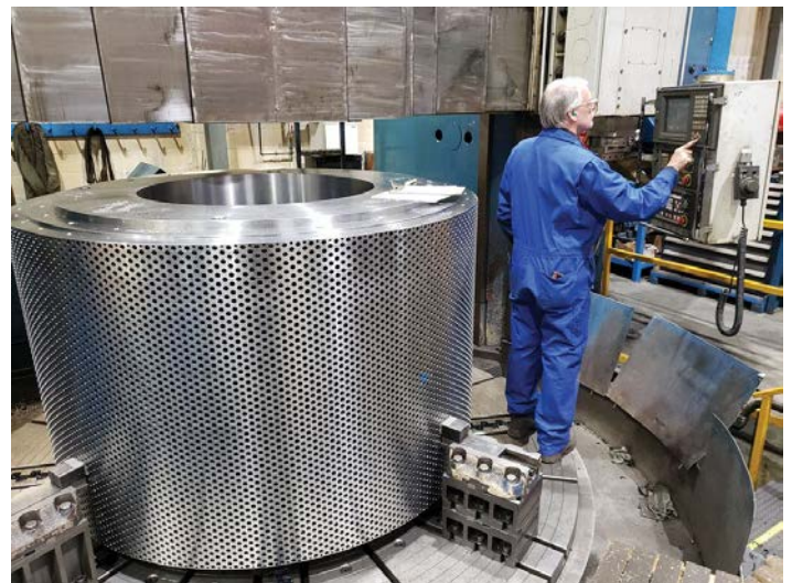
An operator prepares to finish machine the bore on this heavy metal part to specification on the shop’s vertical CNC boring mill.
