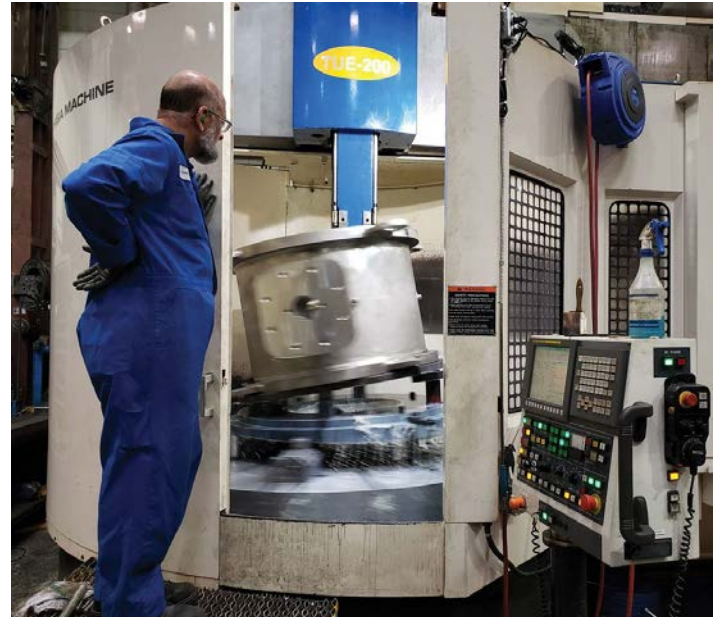
An operator machines valve seats to tight tolerances on the shop's latest acquisition, a Toshiba TUE-200(S) vertical lathe with live tooling.
