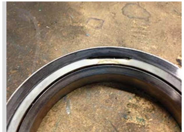
Figure 3. The product flowing through the valve was hitting against the seat face inserts when the valve was in a partially open position, which then caused a seat leak path when the valve was fully closed."
