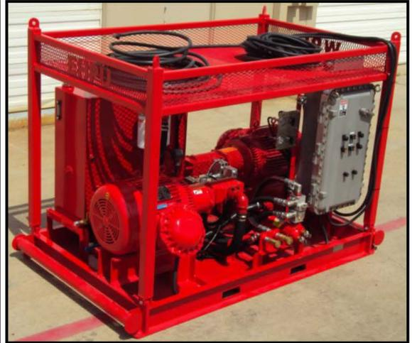
**Description:** Skid mounted, electric hydraulic power unit, for operation of casing and tubing tongs
