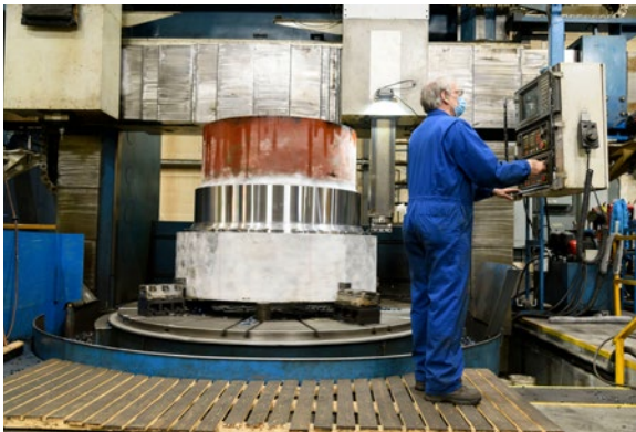
Universe Manufacturing Division: Machining a large part to size on a CNC Vertical Boring Mill, Rolf Reukema.
