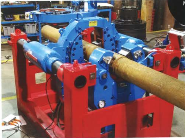
Torquing Pipe - Universe 9.625 Bucking Unit.
